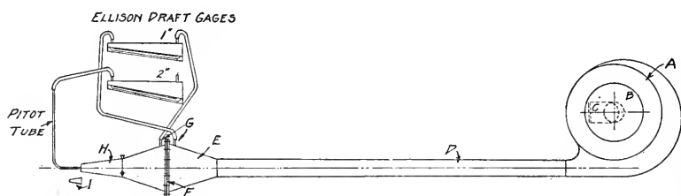
FIG. 1. ASSEMBLED APPARATUS FOR TESTING FILTERS
